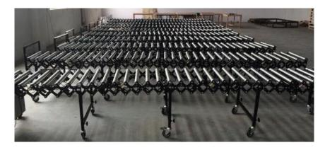
▲ **Conveying surface:** Conveying surface is composed of Polyvee-belt driven Dia.
